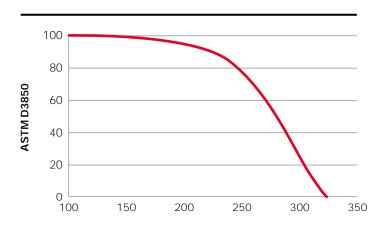
Additive volatility can infuence lubricant performance characteristics. Thermogravimetric analysis (TGA) of Naugalube® 750 demonstrates its excellent thermal and oxidative stability.
