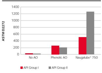
RPVOT (Rotating Pressure Vessel Oxidation Test) performance testing shows superior antioxidant properties performance over the phenolic antioxidant in both Group I and Group II turbine oil formulations with a clear and significant performance boost achieved with Naugalube® 750 in the Group II based oil.
